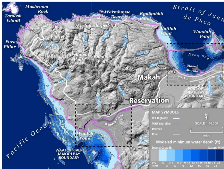
Figure 28: Overview of modeled minimum water depths from the tsunami generated by the Cascadia subduction zone earthquake scenario. Tidal datum: Mean Low Water. Model resolution: 1/9th arc-second (3 m).
